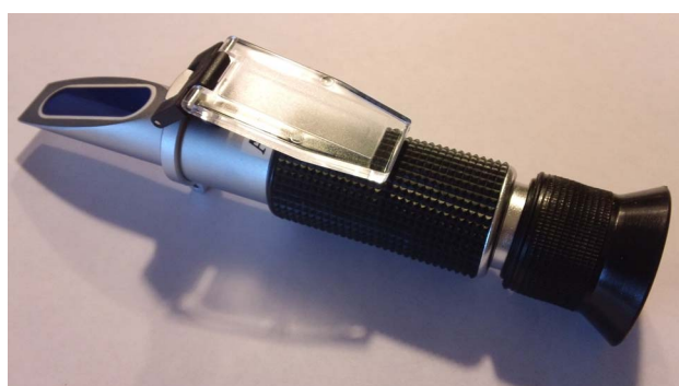
Figure 1. Hand-held optical refractometer.
